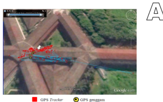
Gambar 5. Plot hasil uji coba stasiuner pada area tertutup Figure 5. Plot of stationary test results in a closed area
